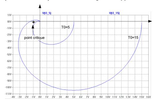
$$\begin{split} T_{bo}(j\omega) &= \frac{T_0}{(1+j\omega/\omega_1)*(1+j\omega/\omega_2)*(1+j\omega/\omega_3)} \\ &= \text{avec:} \\ \omega_1 &= 100, \omega_2 = 200 \, \text{et } \omega_3 = 300 \\ T_0 &= 5 \, \text{ et } T_0 = 15 \end{split}$$
